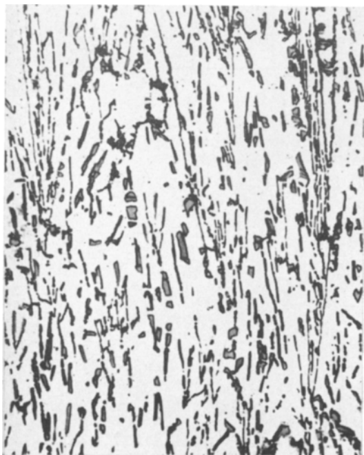
Figure 9 Longitudinal section ( \times 430 ) of a tensile sample taken from a 4 mm diameter specimen, after tensile testing, showing multiple fracture of the boron fibres. The sample was grown at 7.08 \times 10^{-2} mm sec. ^{-1} .
